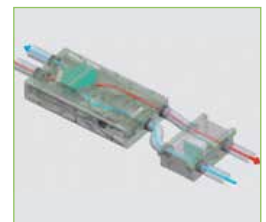
Activation of photocatalysis thanks to the UV lamp and re-introduction of purified air.
